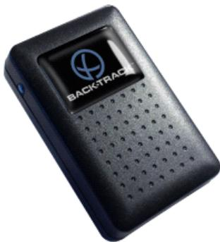
BACK-TRACK™ movement sensors were used in this study. BACK-TRACK™ devices are matchbox sized, sophisticated motion sensing and data collection units, used primarily in manual handling contexts<sup>64</sup>. As well as data collection, it has a vibration facility which can be programmed to respond to various conditions; for example inactivity of a certain duration; stooping etc.
